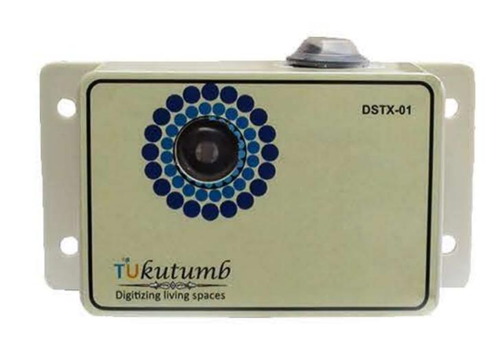
SENSES THE ENVIRONMENT AND SENDS COMMANDS TO COMPATIBLE SMART INTELLIGENT ELECTRICAL SWITCHES IN ITS VICINITY.
